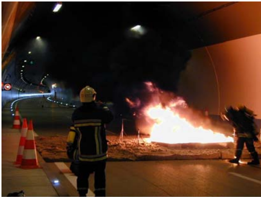
Test of fire-detection and ventilation, source: STUVA
